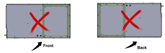
Multiple air handlers configured for installation with a single Rinnai tankless water heater or boiler is prohibited.
