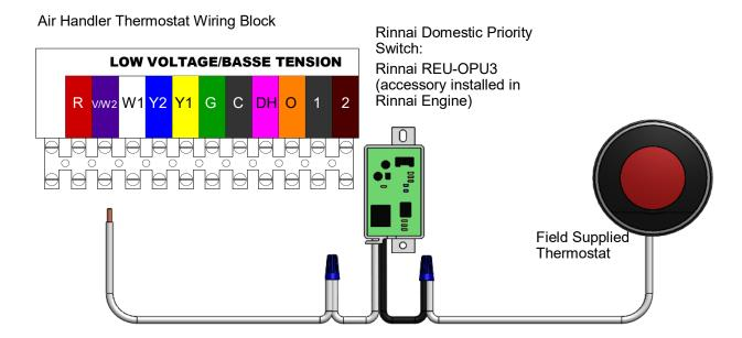
Connections to the Air Handler PC Board. Other thermostat wires removed for clarity.
