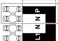
P = Pump Line Wire Terminal N = Pump Neutral Terminal
