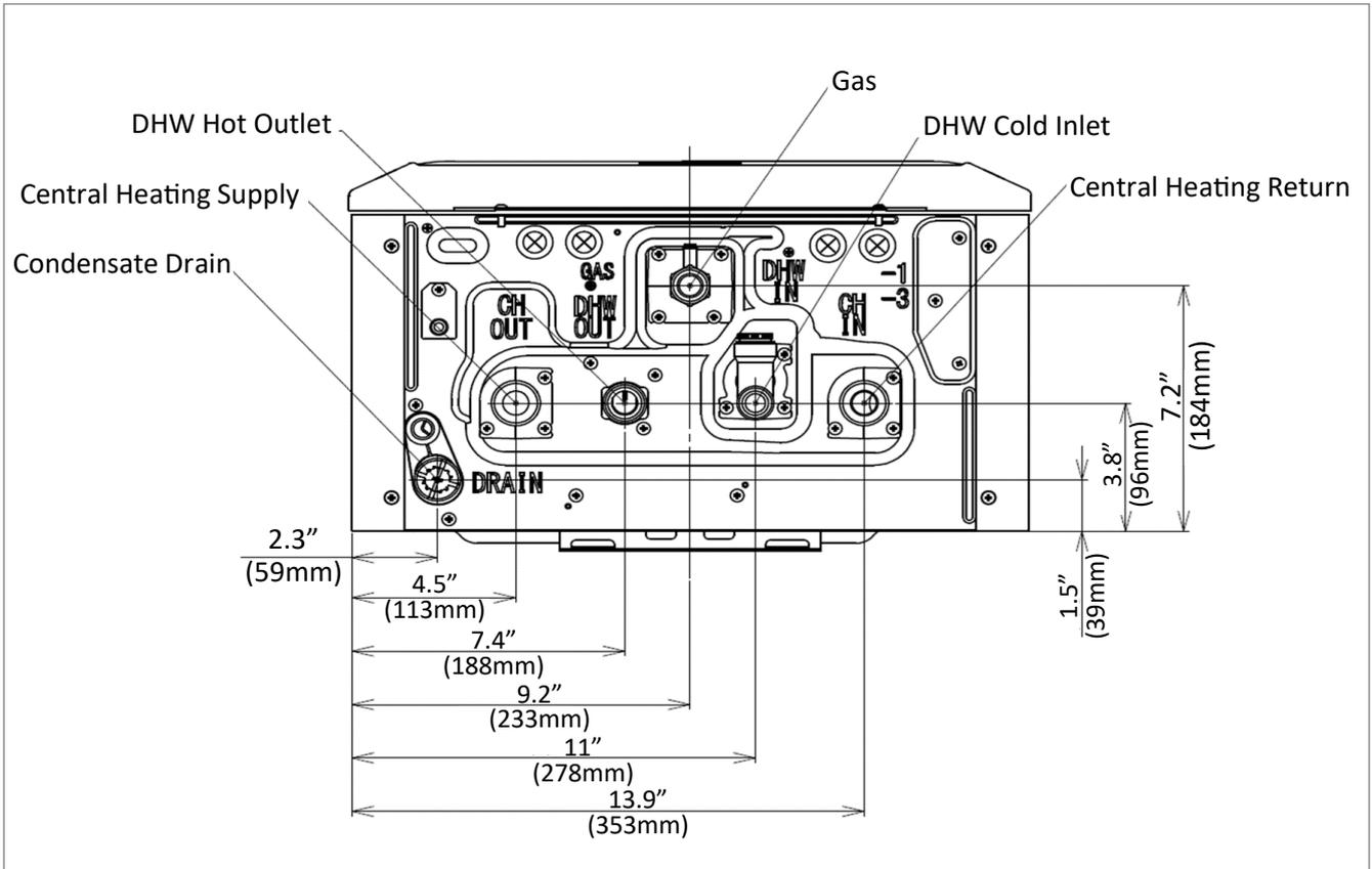
Figure 6: Supply Connections
