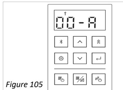
6. Press the ▲ (Up) or ▼ (Down) arrows to select a parameter setting number. Then, press the **Select** button.
