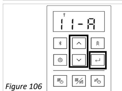
7. Press the ▲ (Up) or ▼ (Down) arrows to change the selection for the setting number (such as 11-A or 11-b). Then, press the **Select** button.
